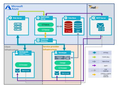
Note 1: Communication between GTServer and its clients (GTAnswer, GTWeb, Automation) uses a proprietary protocol at the Application layer (Internet Protocol Suite model or OSI model). The SSL/TLS protocol can be used to secure communications.
